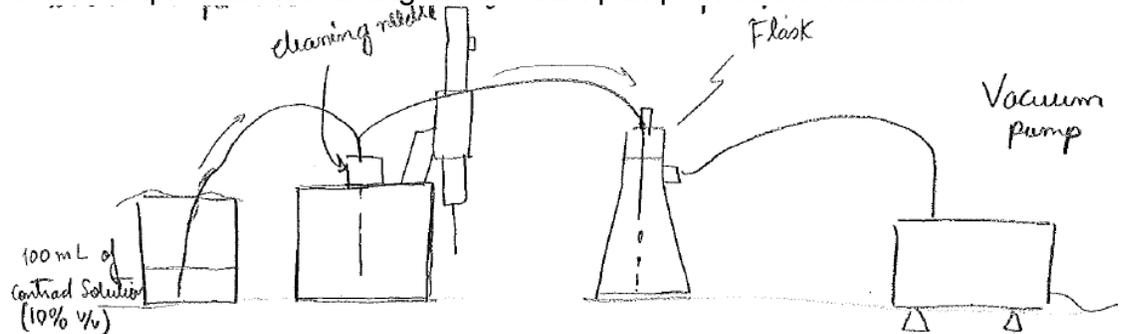
6. Repeat steps 3 and 4 with 150 mL ddH<sub>2</sub>O and then with 200 mL ddH<sub>2</sub>O. Leave water in the sample cell.
