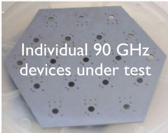
90 GHz Prototype wafer
